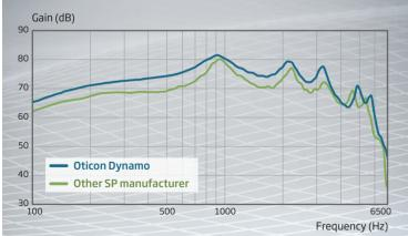
Full-On Gain measurements performed in technical settings according to IEC-60118 (711 coupler). Oticon Dynamo (blue) and other manufacturer (green). Both super power devices are size 13 battery.
